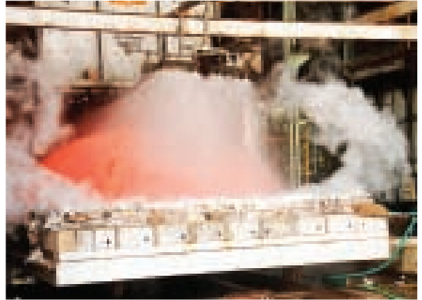
Solution Annealing of 4.5 meters dia. SS Dishend
