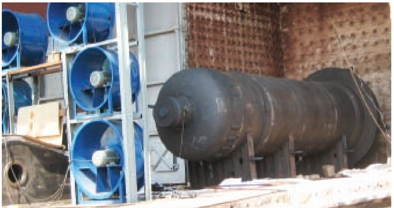
Forced Air Cooling SS claded Vessel
