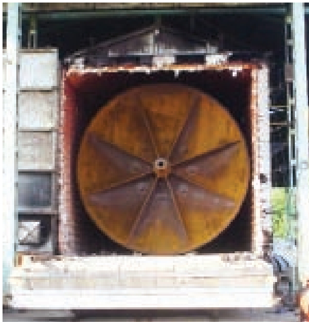
14 feet dia. MG roller PWHT
