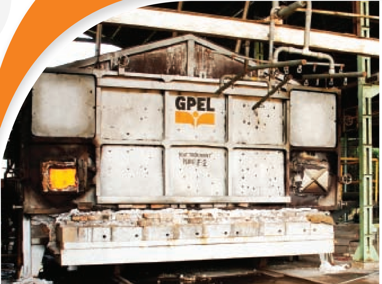
F2 Furnace: Annealing of High chrome casting in Progress
