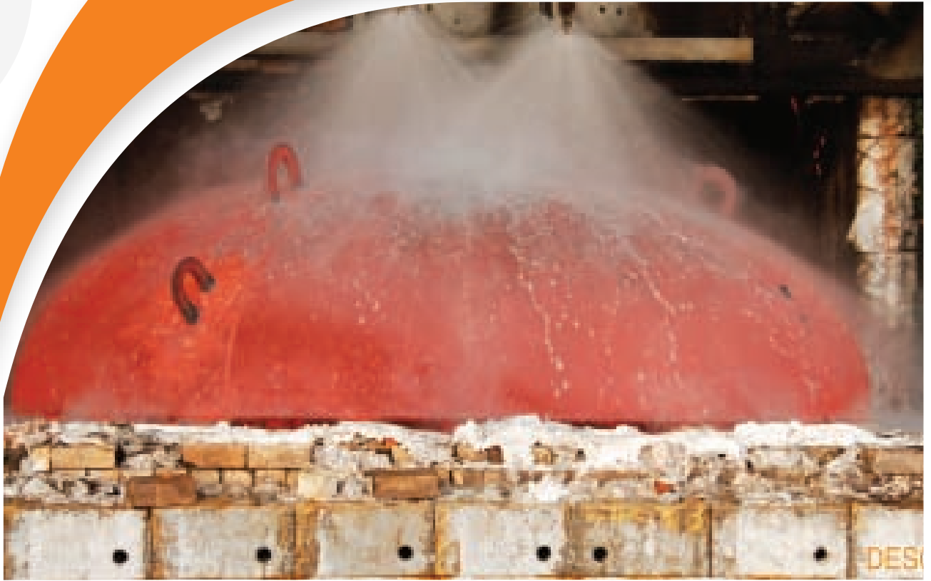
Solution annealing 4.5 dia. SS Dished end
